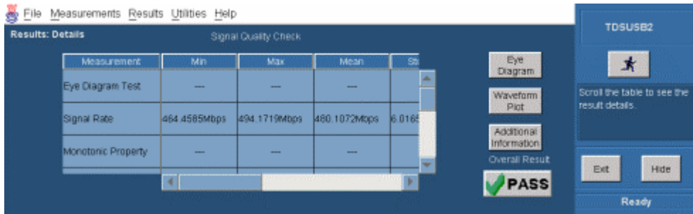
Figure 44: Results details for a High Speed Signal Quality Measurement
